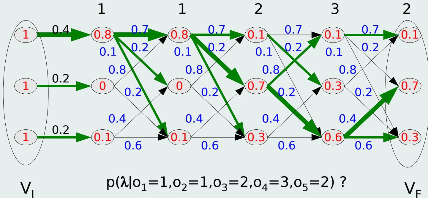
$$p(o_1, o_2, \dots, o_T | \lambda) = \sum_{V} p(s_1) \cdot \prod_{k=1}^T p(o_k | s_k) \cdot p(s_{k+1} | s_k)$$
